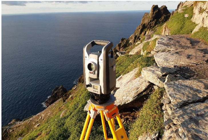
FIGURE 3– VX TOTAL STATION
