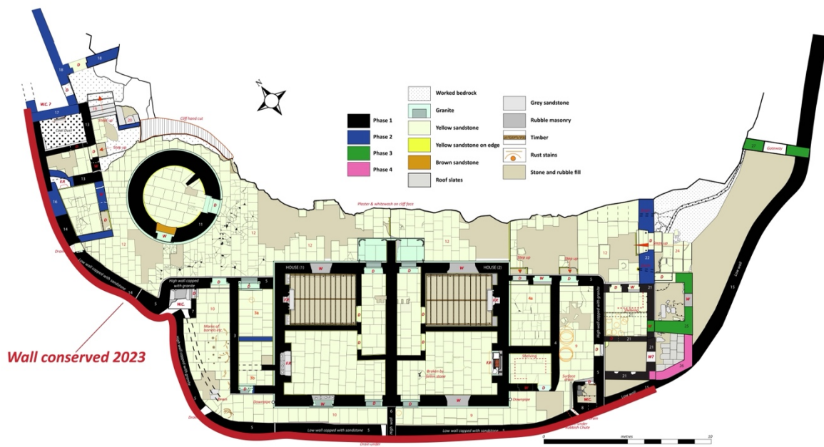
Fig. 1. Plan of the Upper Lighthouse station showing the part of the perimeter wall conserved in 2023.
