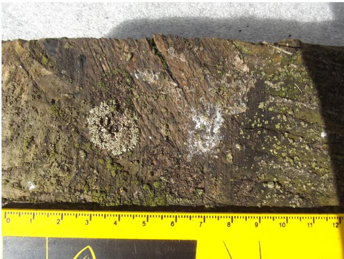
Figure 2. Surface growth of algae and lichen.
