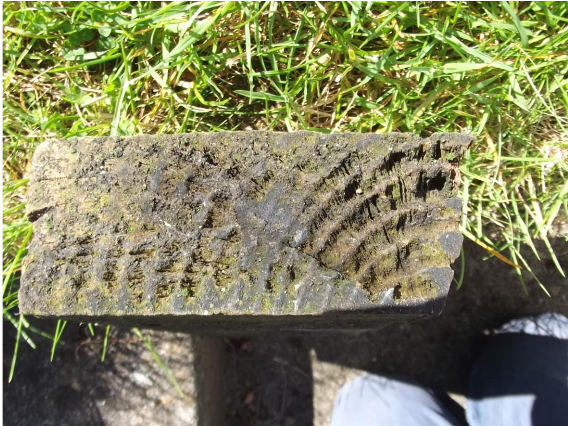
Figure 1. End-grain, showing wide rings and erosion of the early wood.
