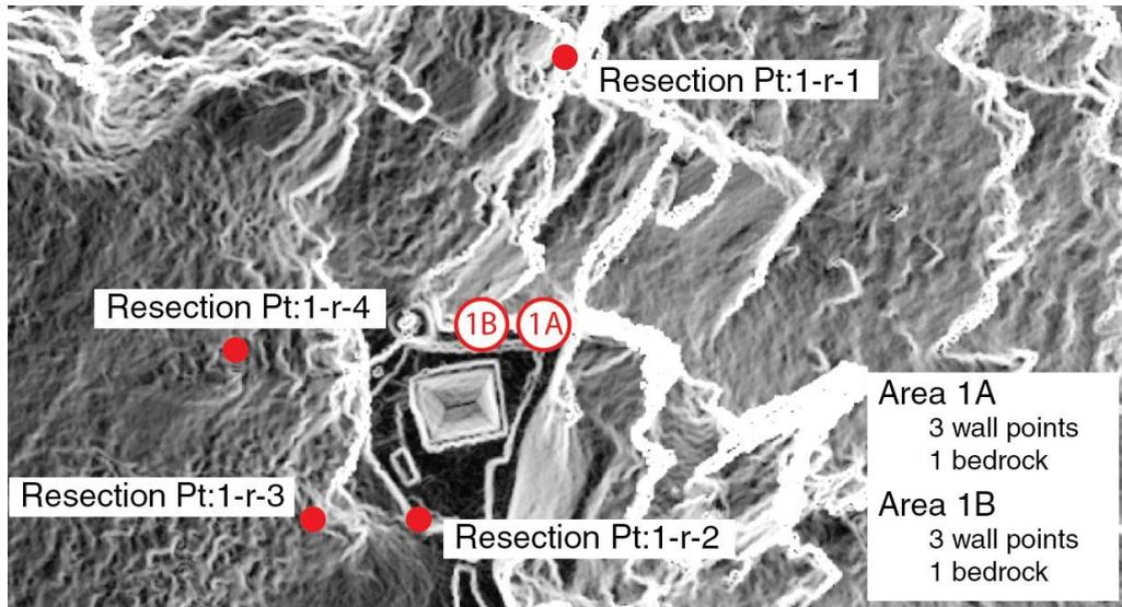
FIGURE I - PLAN LOCATING RESECTION CONTROL NETWORK FOR AREA 1
