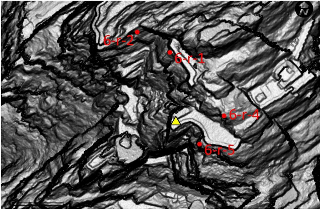
FIGURE X PLAN LOCATING RESECTION CONTROL NETWORK FOR AREA 6
