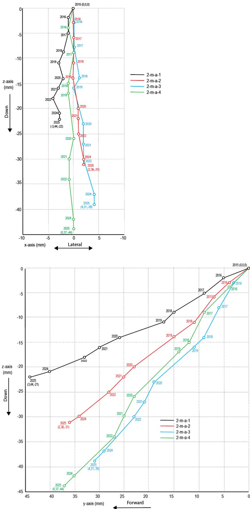
FIGURE 12 – AREA 2, LINE A, LATERAL AND FORWARD MOVEMENT 2D GRAPHS
