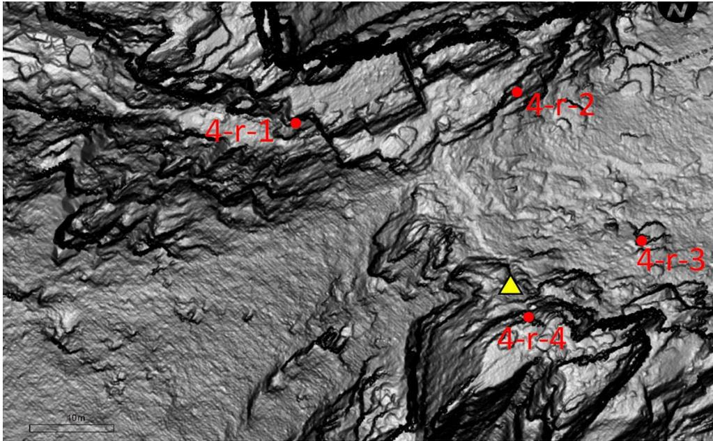
FIGURE VI - PLAN LOCATING RESECTION CONTROL NETWORK FOR AREA 4
