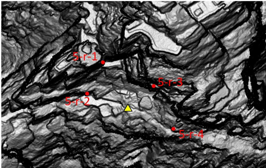
FIGURE VIII - PLAN LOCATING RESECTION CONTROL NETWORK FOR AREA 5
