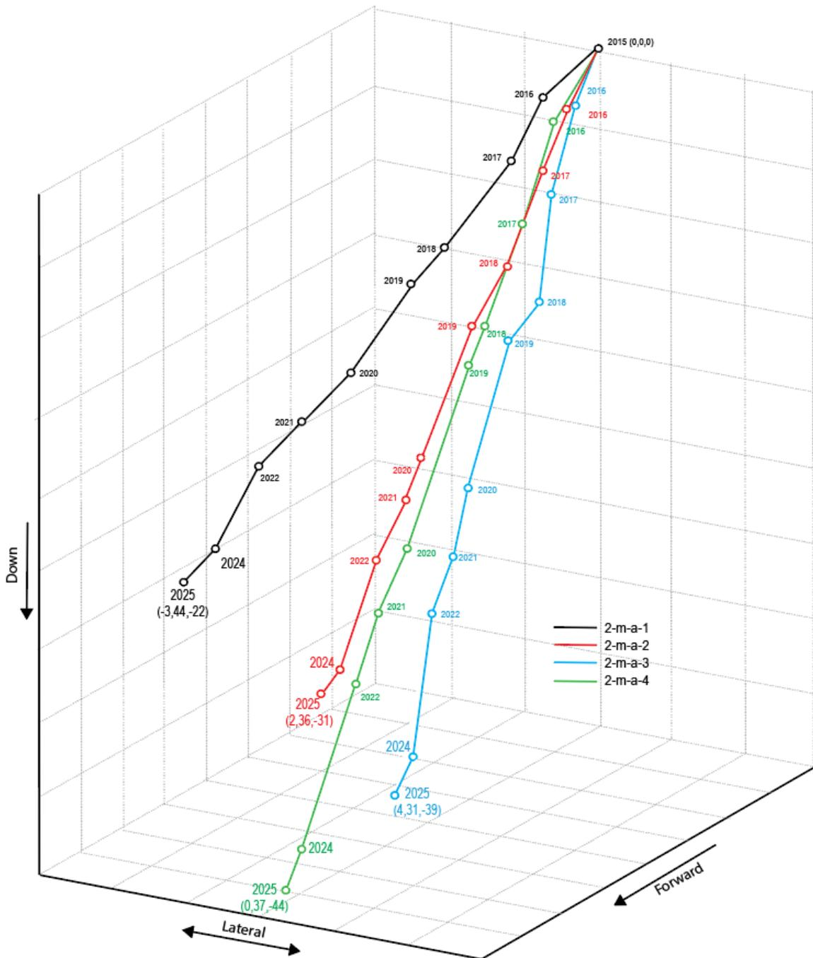
FIGURE 11 - AREA 2, LINE A, SCHEMATIC 3D DIAGRAM OF MOVEMENT OVER DURATION OF THE MONITORING SURVEY OF EACH SURVEY MARKER
