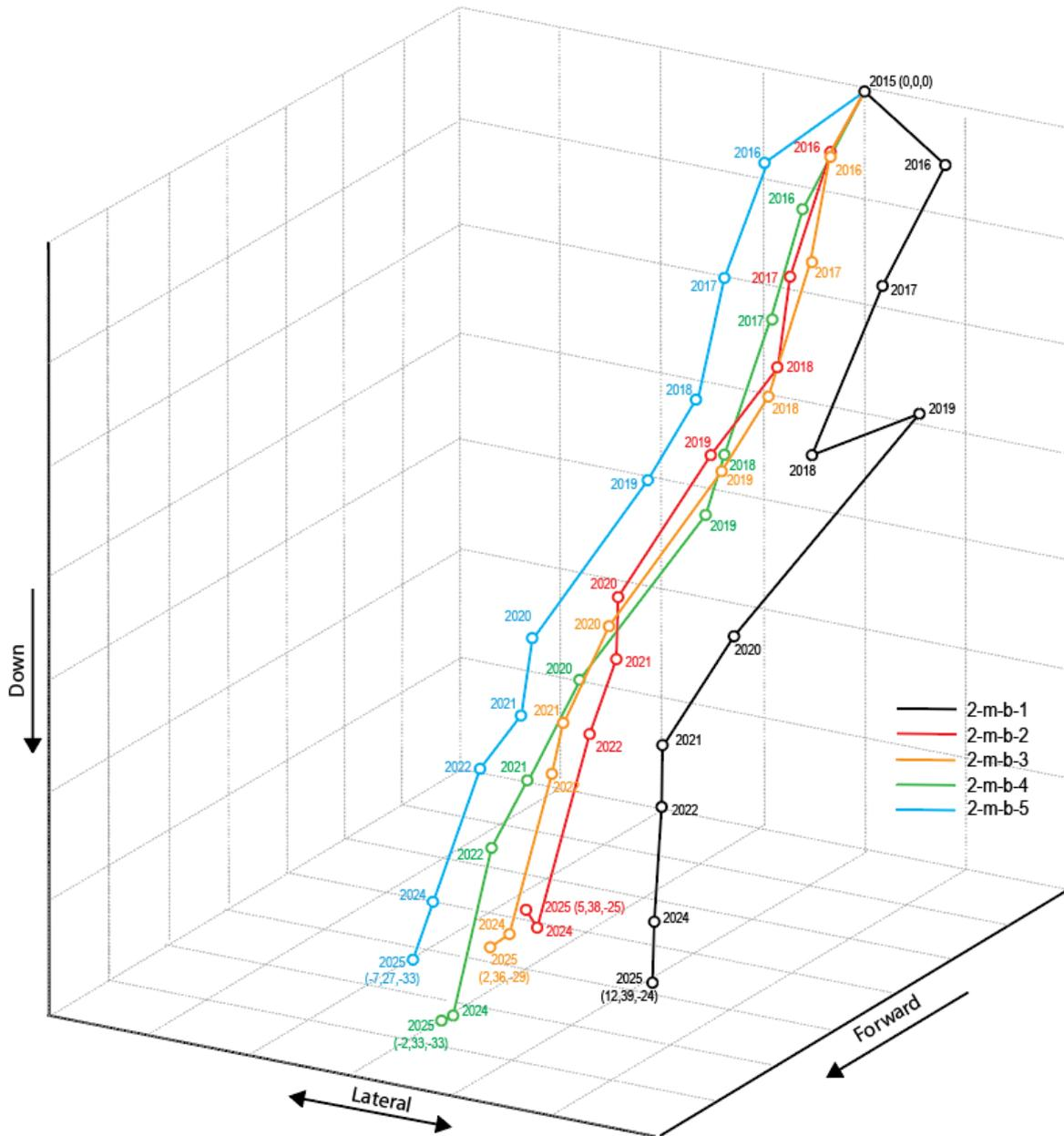
FIGURE 13- AREA 2, LINE B, SCHEMATIC 3D DIAGRAM OF MOVEMENT OVER DURATION OF THE MONITORING SURVEY OF EACH SURVEY MARKER
