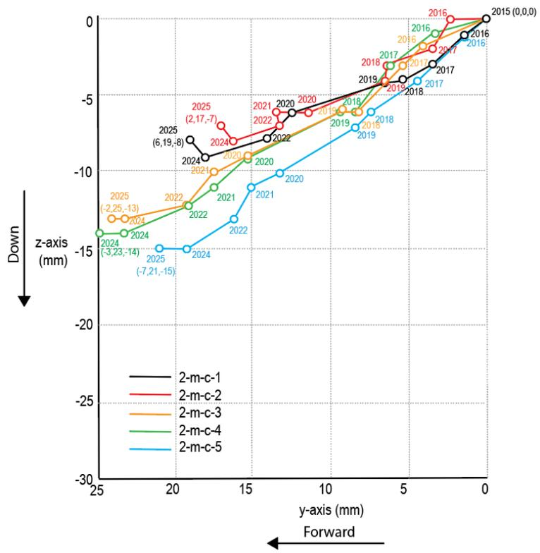
FIGURE 16 - AREA 2, LINE C, LATERAL AND FORWARD MOVEMENT 2D
