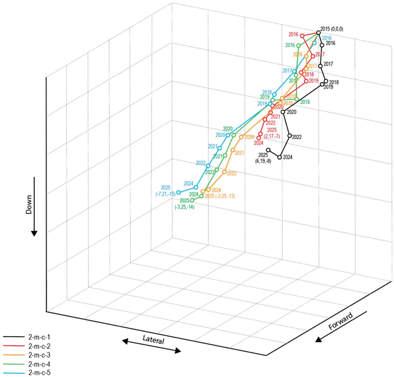
FIGURE 15 - AREA 2, LINE C, SCHEMATIC 3D DIAGRAM OF MOVEMENT OVER DURATION OF THE MONITORING SURVEY OF EACH SURVEY MARKER
