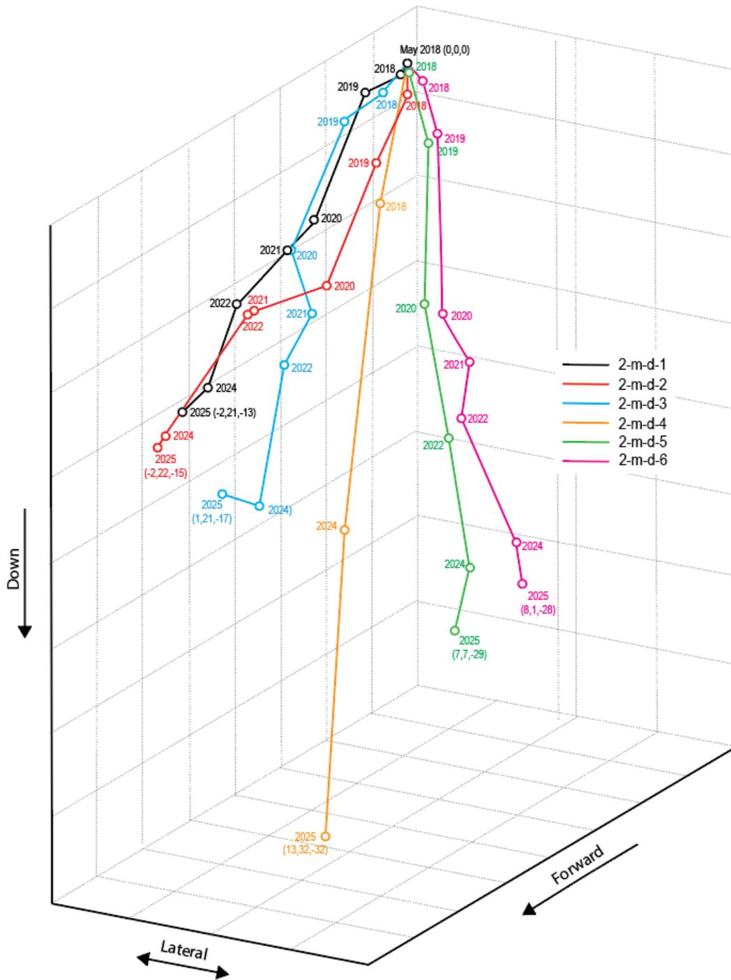
FIGURE 17- AREA 2, LINE D, SCHEMATIC 3D DIAGRAM OF MOVEMENT OVER DURATION OF THE MONITORING SURVEY OF EACH SURVEY MARKER
