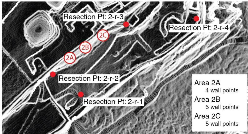
FIGURE II - PLAN LOCATING RESECTION CONTROL NETWORK FOR AREA 2
