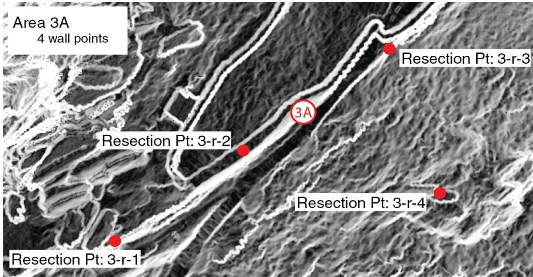
FIGURE IV - PLAN LOCATING RESECTION CONTROL NETWORK FOR AREA 3
