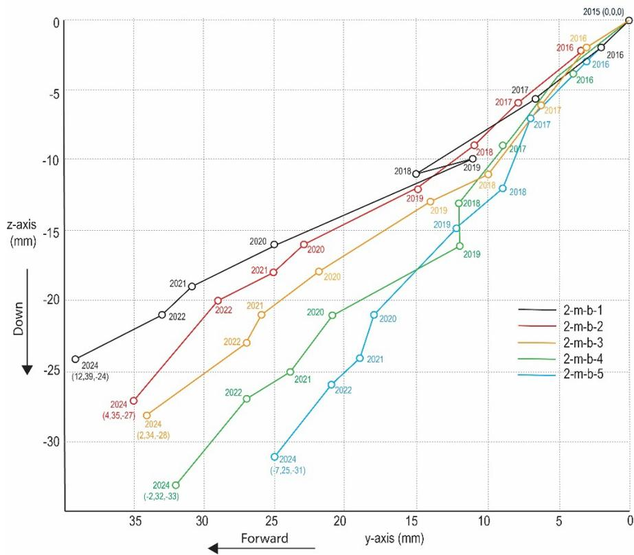
FIGURE 14 - AREA 2, LINE B, LATERAL AND FORWARD MOVEMENT 2D GRAPHS
